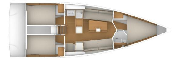
Simple, comfortable and multi-purpose, the First 36 interior was developed around three-cabin cruising functionality. Its most notable feature is the large central fridge (with a removable cutting board), making this sailboat's galley the largest of her class. A corridor created together with the foldable and removable table helps sailors move around the saloon safely and offers stacking possibilities.
